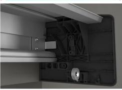
5.7 Insert the belt in the pulley motor drive unit, slide it and pass it around the transmission unit and fix to carriage with the proper springs (see the belt attack position, as shown in Chapter 4).
