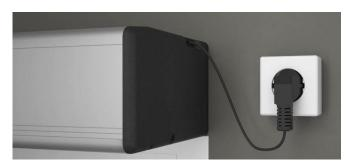
In case there isn't a socket near the automation, to perform the connection to the power supply in the following manner: drill the aluminum profile in the upper part or in the rear wall fixing, protect the passage of the power cord through membrane grommets or cable glands (not supplied by us) to eliminate sharp edges that might damage the power cable, and connect the cable to the power supply.
