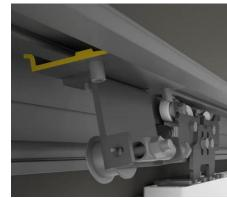
5.5 Insert the carriages in front of the drive unit profile, and adjust the upper wheel, so you do not let them get out of the rail profile [104] In case of 2-leaves automation, also add the carriages for the left leaf.
