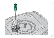
No Remove the cover of the operator and the cable clamp. Slide out the electrical cable and route into the through-hole.
