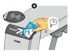
**the** Press the master card against the sensor for longer than three seconds to access the programming mode.
