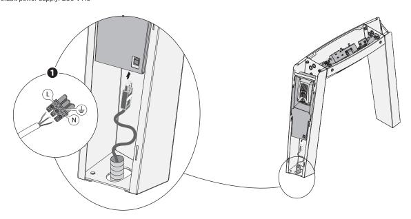
To switch to 120 V current, unplug the power supply and control unit to access, via the lateral hole, the selection lever, and flick it upwards. 23
