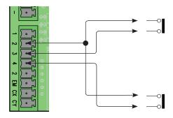
**Command for counter-clockwise operation** (NO), with local and remote device. For counter-clockwise release of the turnstile
